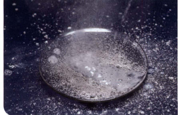
Calcium hydride (CaH 2 ) reacting with water, releasing hydrogen gas (H 2 ).
