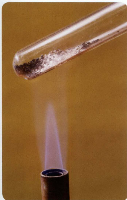
This photo shows a decomposition reaction in action: 2\text{Ag}_2\text{O} \rightarrow 4\text{Ag} + \text{O}_2 .
