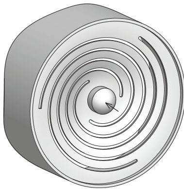
Figure 8-6 Triple spiral frictionless flexure for guiding axial displacement.
